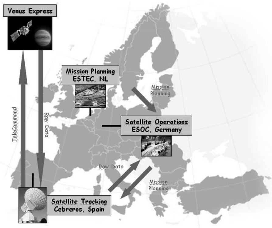
Figure 2. Uplink/downlink data flow.
